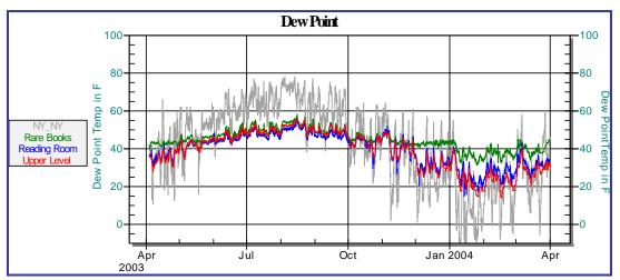
coils and drains away) to wring the moisture out of the air. You can see this dehumidifying effect quite clearly in the graph below.
