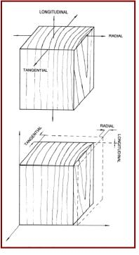
longitudinally. Tangential dimensional change has the highest rate of change due to parallel orientation of microfibrils along the axis of the cell wall. Variations in humidity levels result in dimensional changes -- wood absorbs moisture and swells in high humidity; it releases moisture and shrinks in low humidity.
