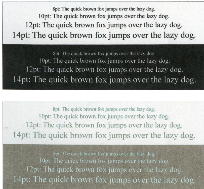
Figure 11. Worst performing text target print; a) before and b) after 12 weeks of exposure to 50 Klux fluorescent light.
