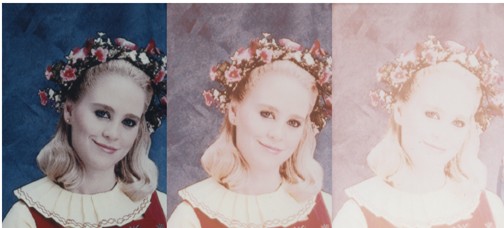
Figure 6. Dye sublimation print in which xenon arc produced more fade than fluorescent light after 12 weeks of exposure to 50 Klux intensity. Unexposed (left), exposed to fluorescent light (center) and exposed to xenon arc light (right).
