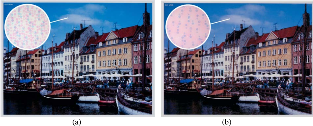
Figure 16: Shows magenta colorant bleed of IJ Dye/Porous-Photo sample. (a) Is the reference image and (b) is the image taken after the bagged period ( \text{NO}_2 pre-dosed).
