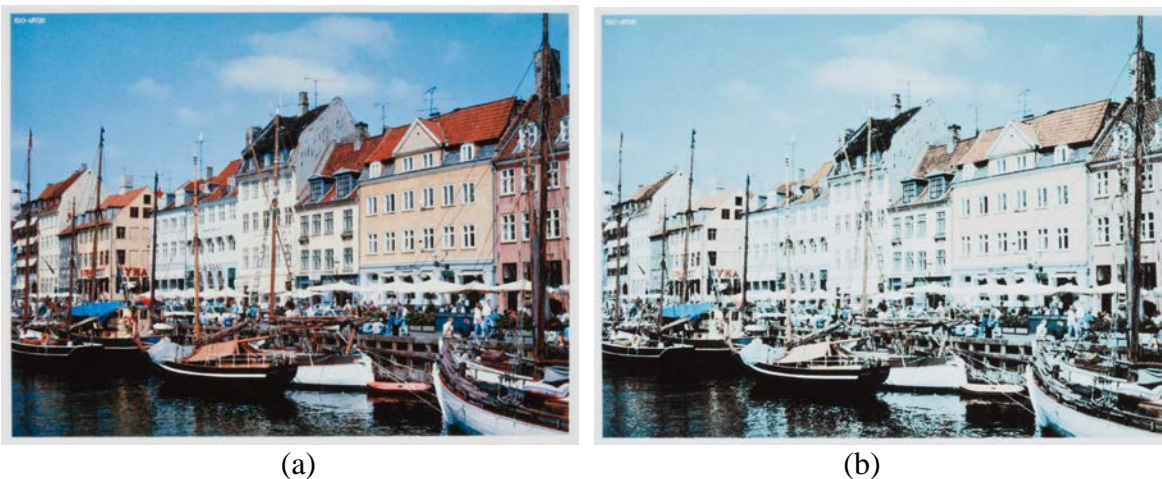
Figure 13: Shows fading of colorants of IJ Dye/Plain-Sized sample. (a) Is the reference image and (b) is the image taken after the bagged period ( O_3 pre-dosed).
