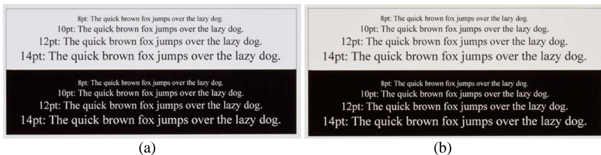
Figure 19: Shows yellowing of digital press sample. (a) Is the reference and (b) is the image taken after the bagged period ( \text{NO}_2 pre-dosed).
