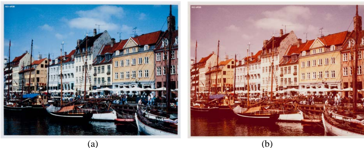
Figure 17: Shows magenta hue shift of the chromogenic sample. (a) Is the reference image and (b) is image taken after the bagged period ( \text{NO}_2 pre-dosed).
