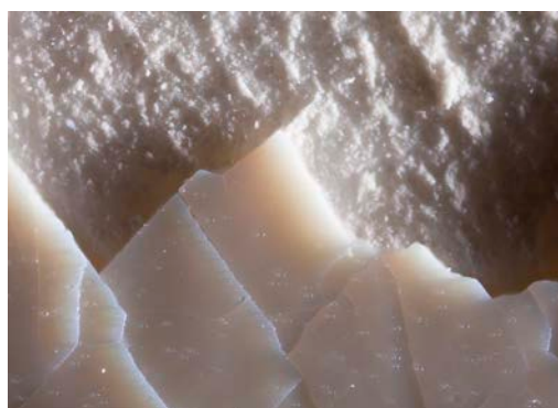
Figure 9: Shows delamination of a small area (100x)
