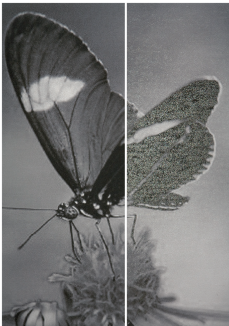
Figure 7. Even high-quality interleaving papers could cause colorant smear or polishing/burnishing of the image
