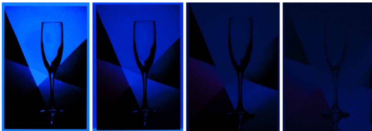
Figure 11 Inkjet dye print on photo-porous paper after exposure to 50 klx of xenon arc light for 6 weeks in different framing configurations, viewed under UV lamp to show degrees of OBA protection conveyed by UV glass and plain glass. Unexposed – left; exposed with UV glass – center-left; exposed with plain glass – center-right; and exposed without glazing – right.
