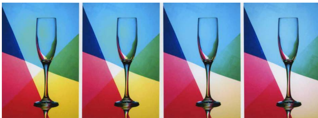
Figure 6 Inkjet pigment print on photo-porous paper after exposure to 50 klx of xenon arc light for six weeks in different sealed framing configurations. Unexposed – left; exposed with UV glass – center-left; exposed with plain glass – center-right; and exposed without glazing – right. The use of UV glass noticeably preserves the print’s weakest colorant (yellow).
