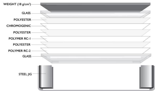
Figure 2: Jig stacking order
