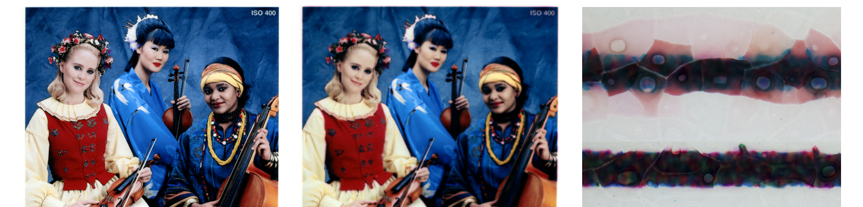
Humidity-induced bleed results in loss of detail, image sharpness, and color fringing
